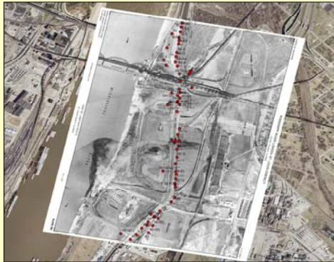
Figure 2. Imagery showing 1956 boring plan and boring locations georeferenced to modern cospatial imagery.
