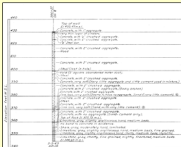
Figure 4. Example boring log illustrating more than 65 ft (19.8 m) junk fill beneath St. Louis Floodwall.
