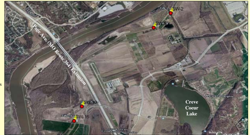
Figure 6. Boring plan illustrating the location of four borings to bedrock as provided by the Howard Bend Levee District.
